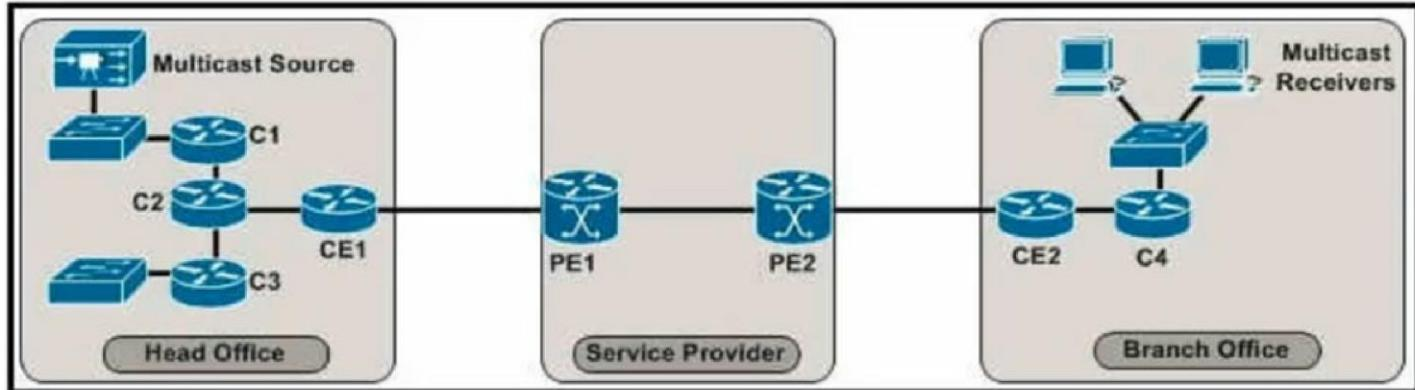
Refer to the exhibit. This enterprise customer wants to stream one-way video from their head office to eight branch offices using multicast. Their current service provider provides a Layer 3 VPN solution and manages the CE routers, but they do not currently support multicast. Which solution quickly allows this multicast traffic to go through while allowing for future scalability?
