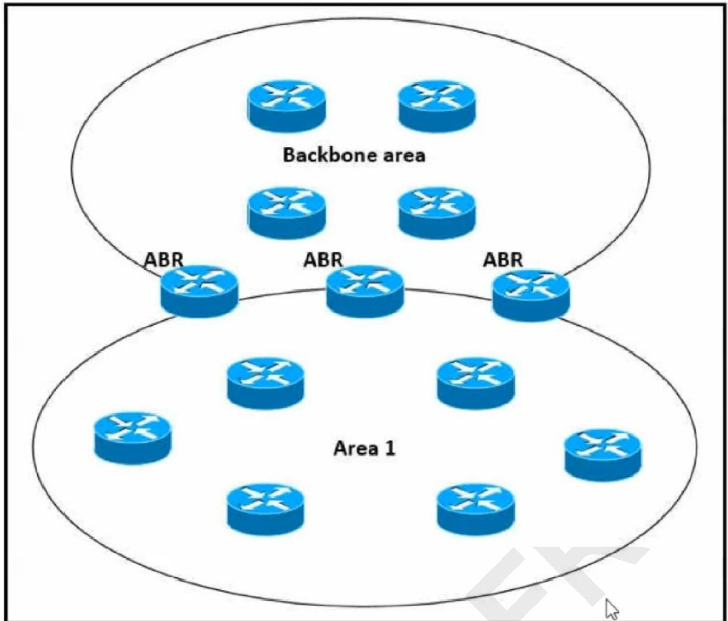
Refer to the exhibit. Which impact of using three or more ABRs between the backbone area and area 1 is true?
