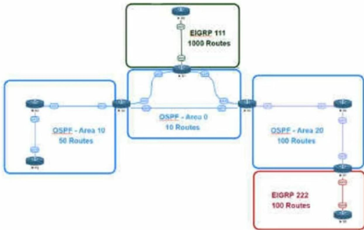
Refer to the exhibit. An engineer is designing a multiarea OSPF network for a client who also has a large EIGRP domain. EIGRP routes are getting redistributed into OSPF. OSPF area 20 has routers with limited memory and CPU resources. The engineer wants to block routes from EIGRP 111 from propagating into area 20 and allow EIGRP 222 routes to flow in. Which OSPF area type fulfills this design requirement?
