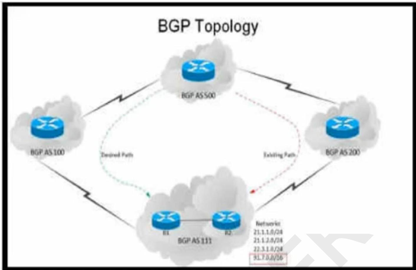
Refer to the exhibit. An engineer has been asked to redesign the traffic flow toward AS 111 coming from AS 500. Traffic destined to AS 111 network 91.7.0.0/16 should come in via AS 100, while traffic destined to all other networks in AS 111 should continue to use the existing path. Which BGP attributes are best suited to control this inbound traffic coming from BGP AS 500 into the 91.7.0.0/16 network?
