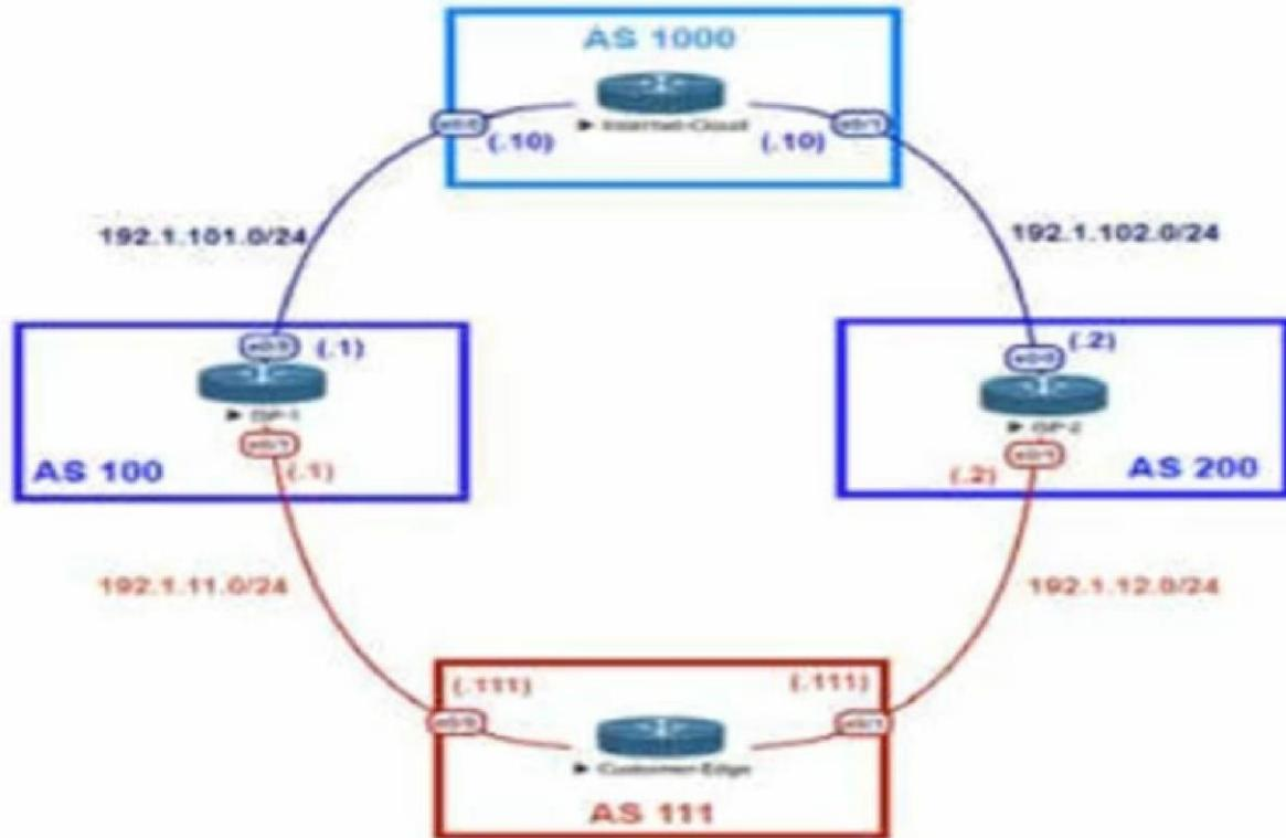
Refer to the exhibit. An engineer is designing the traffic flow for AS 111. Traffic from AS 111 should be preferred via AS 100 for all external routes. A method must be used that only affects AS 111. Which BGP attributes are best suited to control outbound traffic?
