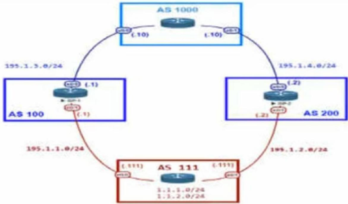
Refer to the exhibit. An engineer is designing the network for a multihomed customer running in AS 111. AS 111 does not have any other ASes connected to it.
