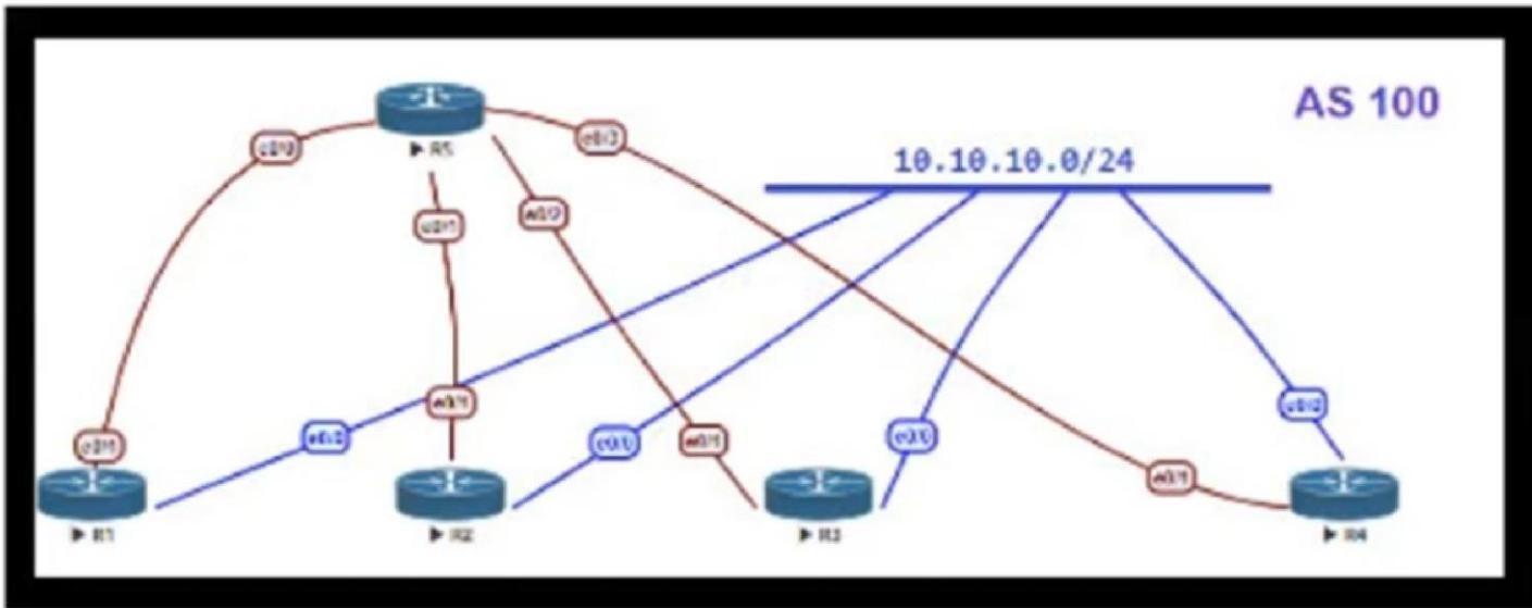
Refer to the exhibit. OSPF is running as the IGP to provide reachability to all AS100 networks. R3 and R4 are the current ABRs at the boundary of OSPF Area0 and Area1. Now BGP must be deployed within AS100 because it will be receiving Internet routes from its eBGP peers (the service provider) connected to R1 and R2. What is an optimal solution for this deployment to configure BGP relationships and redistribute BGP learned routes into OSPF?
