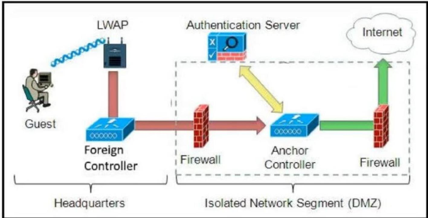
Refer to the diagram. Which solution must be used to send traffic from the foreign wireless LAN controller to the anchor wireless LAN controller?
