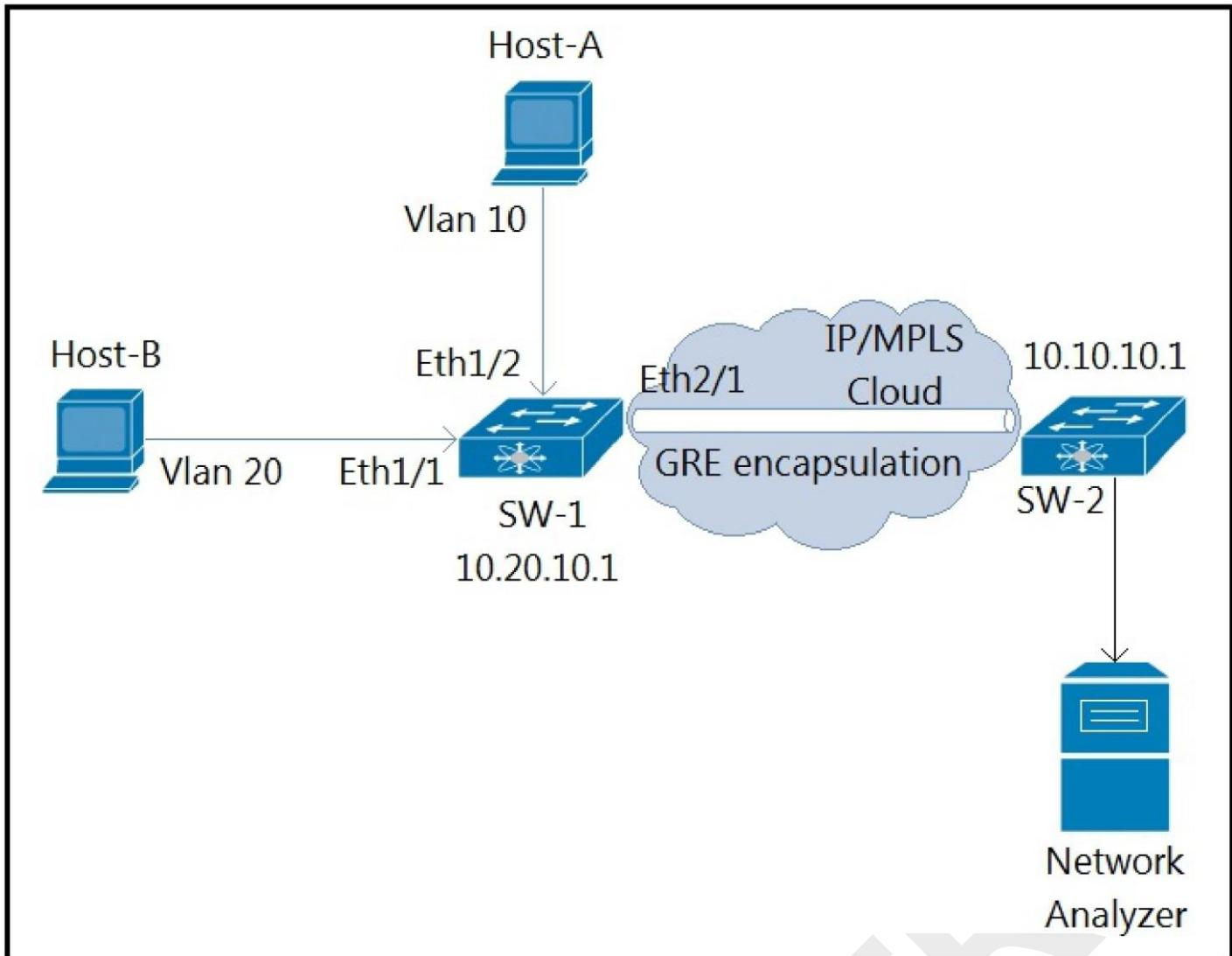
Refer to the exhibit. An engineer monitors ingress traffic from Host-A and all traffic for VLAN 20 from Host-B. Which configuration must be implemented to monitor and export traffic to Network Analyzer?
