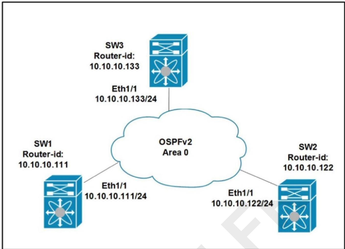
Refer to the exhibit. All switches are configured with the default OSPF priority. Which configuration should be applied to ensure that the SW2 Cisco Nexus switch controls the LSA floods and advertises the network to the remaining nodes in the OSPFv2 area?
