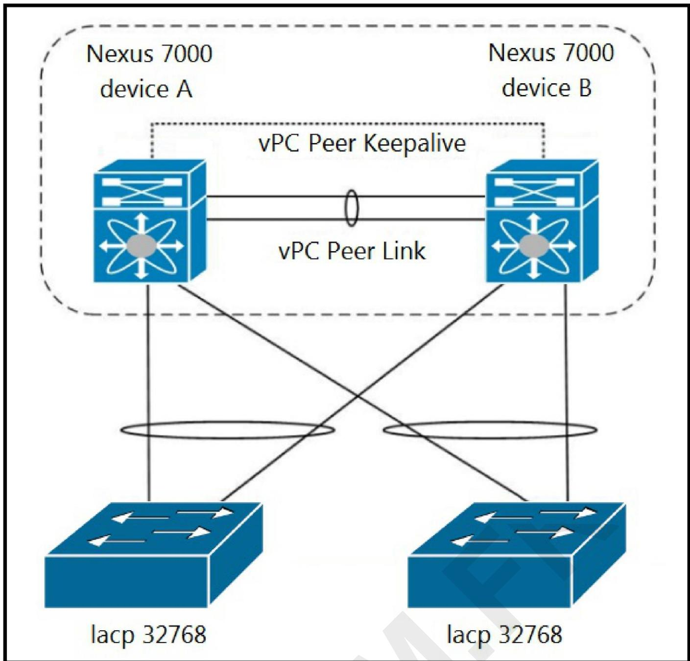
Refer to the exhibit. Which configuration ensures that the Cisco Nexus 7000 Series Switches are the primary devices for LACP?
