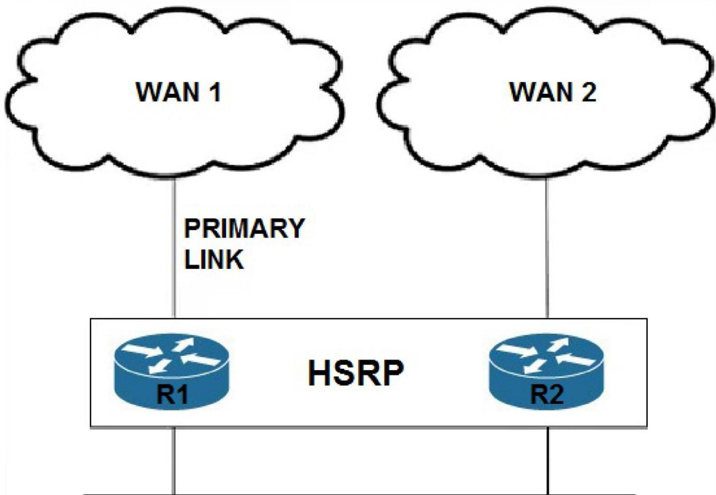
Refer to the exhibit. An engineer must design an automatic failover solution. The solution should allow HSRP to detect a WAN 1 failure and initiate an automatic failover, making router R2 the active HSRP router. Which two solutions should the engineer choose? (Choose two.)
