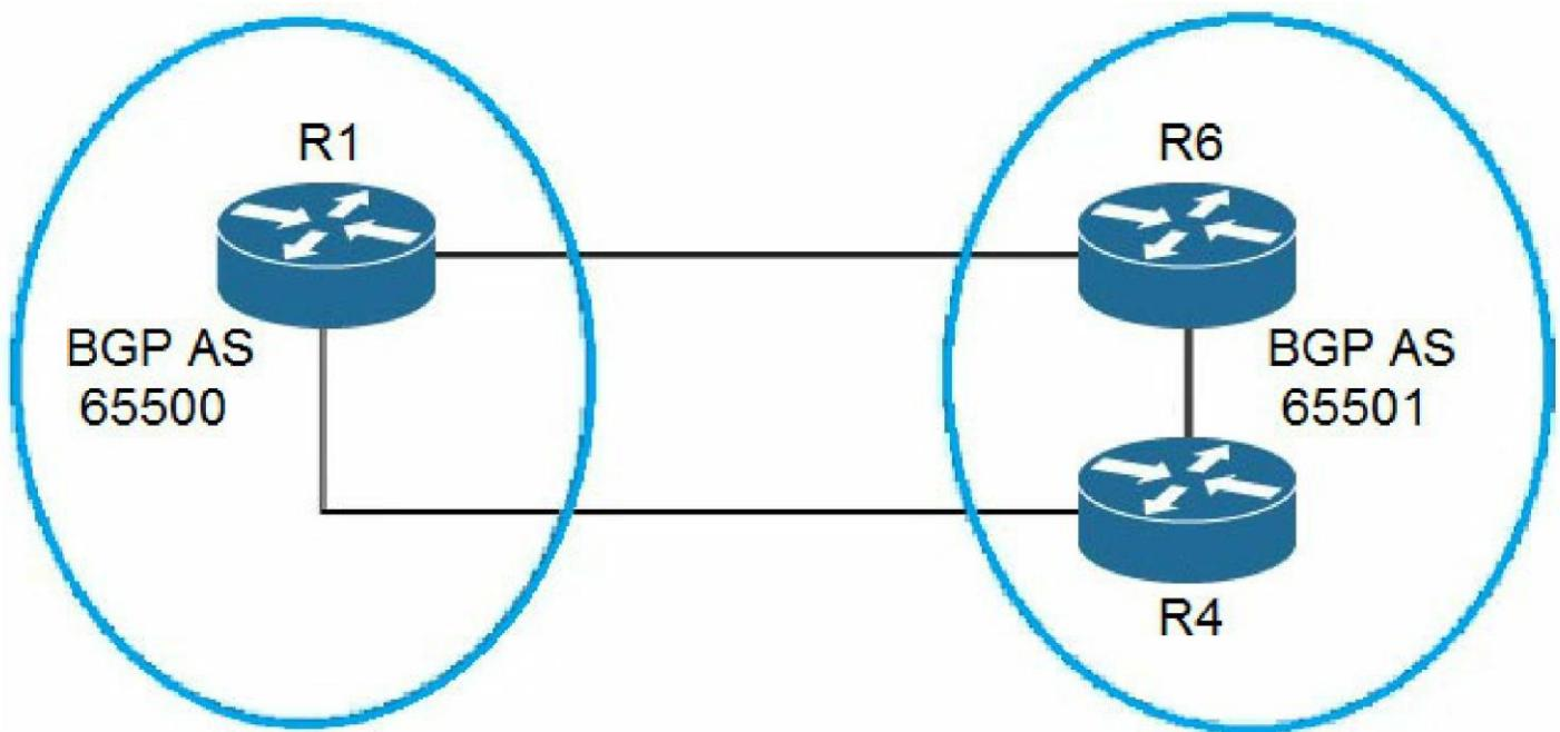
Refer to the exhibit. An architect must design a solution to connect the two ASs. To optimize bandwidth, the design will implement load sharing between router R6 and router R1. Which solution should the design include?
