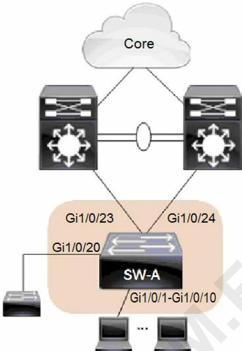
Refer to the exhibit. An architect reviews the low-level design of a company's enterprise network and advises optimizing the STP convergence time. Which functionality must be applied to Gi1/0/1-10 to follow the architect's recommendation?
