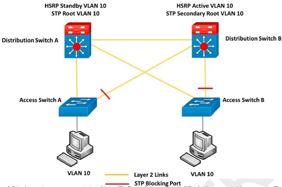
Refer to the exhibit. An engineer must optimize the traffic flow of the network. Which change provides a more efficient design between the access layer and the distribution layer?
