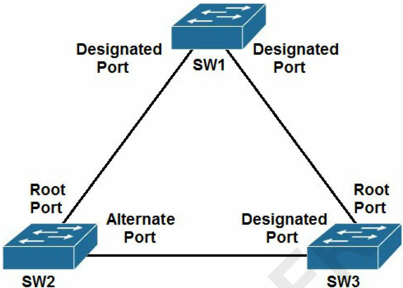
Refer to the exhibit. The connection between SW2 and SW3 is fiber and occasionally experiences unidirectional link failure. An architect must optimize the network to reduce the change of Layer 2 forwarding loops when the link fails. Which solution should the architect include?
