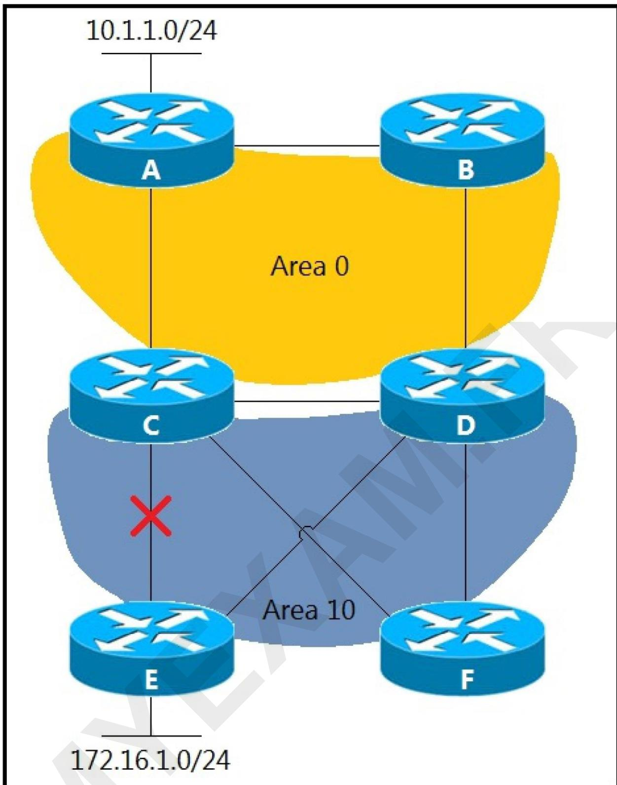
Refer to the exhibit. Area 10 is a regular OSPF area, and networks 10.1.1.0/24 and 172.16.1.0/24 are internal. Which design provides optimal routing between both networks when the link between routers C and E fails?
