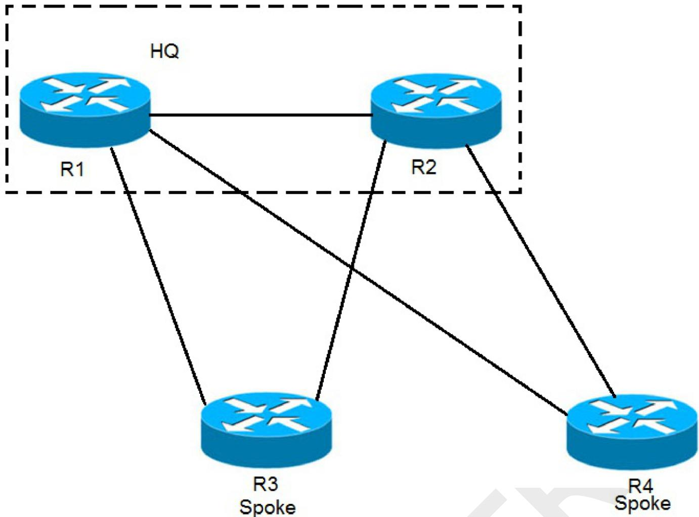
Refer to the exhibit. EIGRP has been configured on all links. The spoke nodes have been configured as EIGRP stubs, and the WAN links to R3 have higher bandwidth and lower delay than the WAN links to R4. When a link failure occurs at the R1-R2 link, what happens to traffic on R1 that is destined for a subnet attached to R2?
