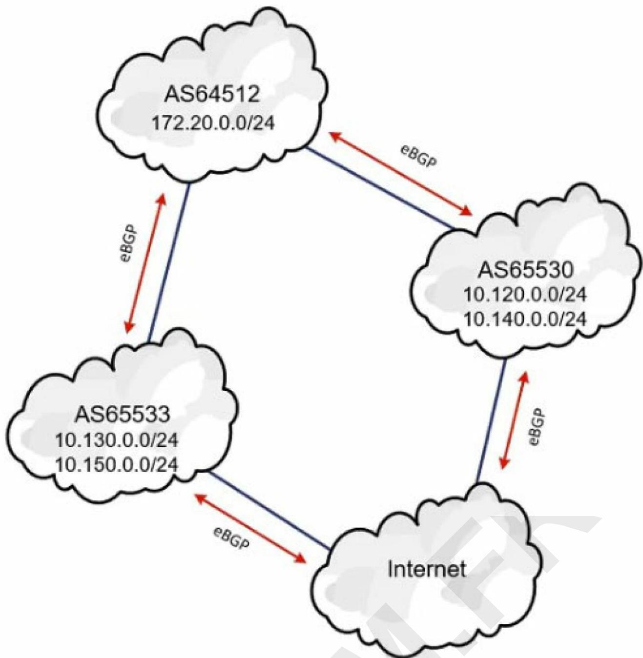
Refer to the exhibit. AS65533 and AS65530 are announcing a partial Internet routing table as well as their IP subnets. An architect must create a design that ensures AS64512 does not become a transit AS. Which filtering solution must the architect choose?
