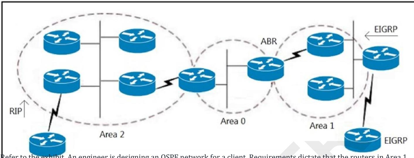
Refer to the exhibit. An engineer is designing an OSPF network for a client. Requirements dictate that the routers in Area 1 should receive all routes belonging to the network, including EIGRP, except the ones that originated in the RIP domain. Which action should the engineer take?
