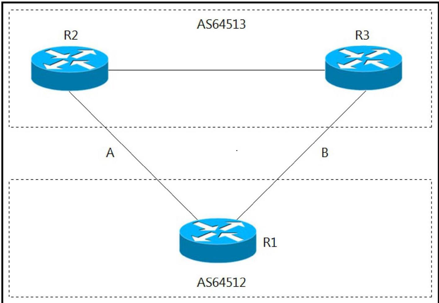
Refer to the exhibit. A network engineer for AS64512 must remove the inbound and outbound traffic from link A during maintenance without closing the BGP session so that there is still a backup link over link A toward the ASN. Which BGP configuration on R1 accomplishes this goal?
