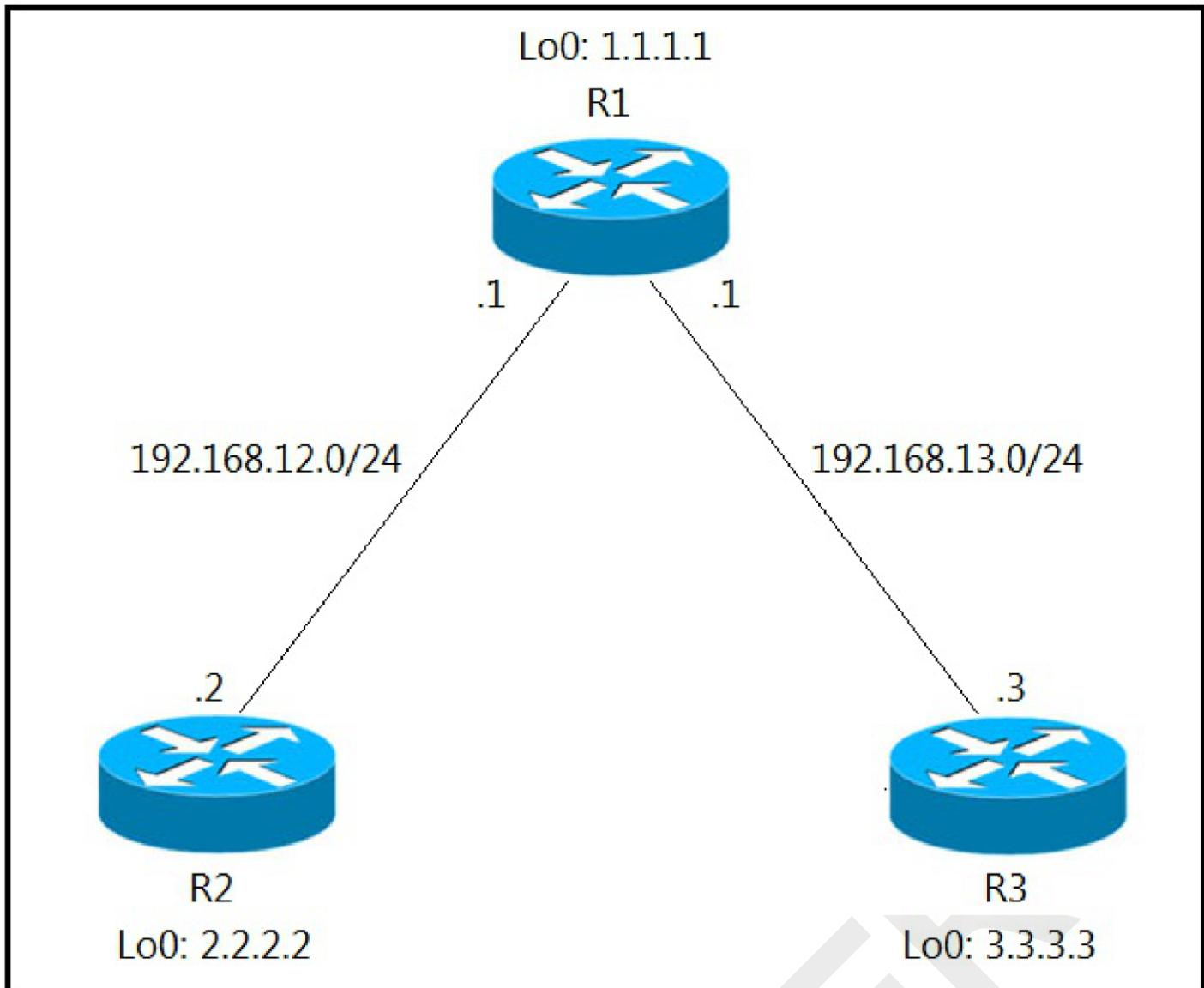
Refer to the exhibit. An engineer has configured R1 as EIGRP stub router. After the configuration, router R3 failed to reach to R2 loopback address.
