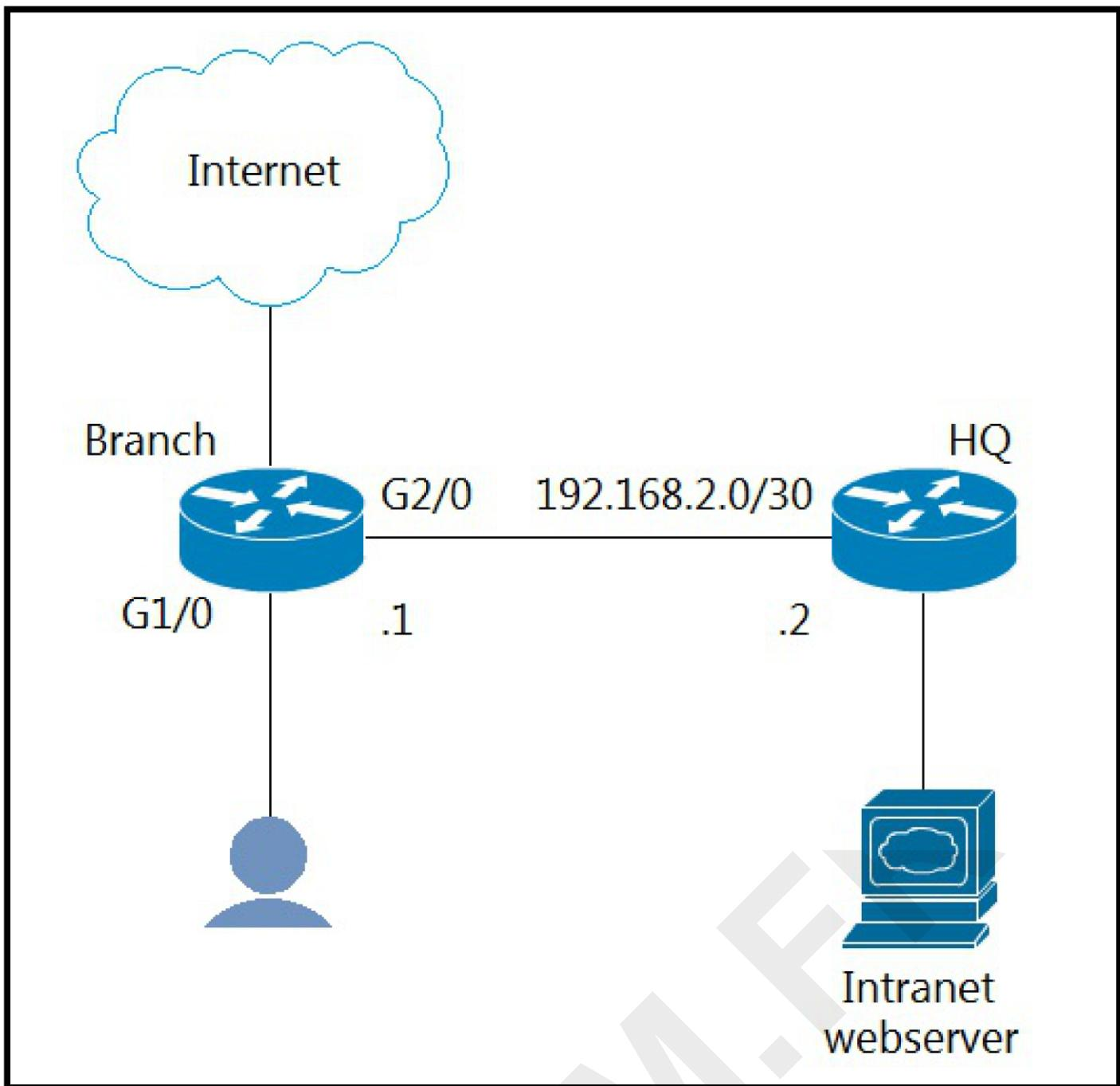
Refer to the exhibit. The branch router is configured with a default route toward the Internet and has no routes configured for the HQ site that is connected through interface G2/0. The HQ router is fully configured and does not require changes.
