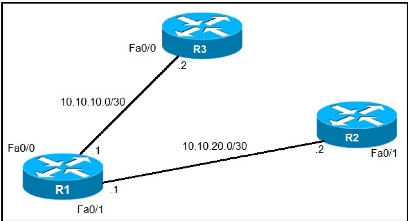
Refer to the exhibit. An IP SLA was configured on router R1 that allows the default route to be modified in the event that Fa0/0 loses reachability with the router R3. Which debug command is used to troubleshoot this issue?
