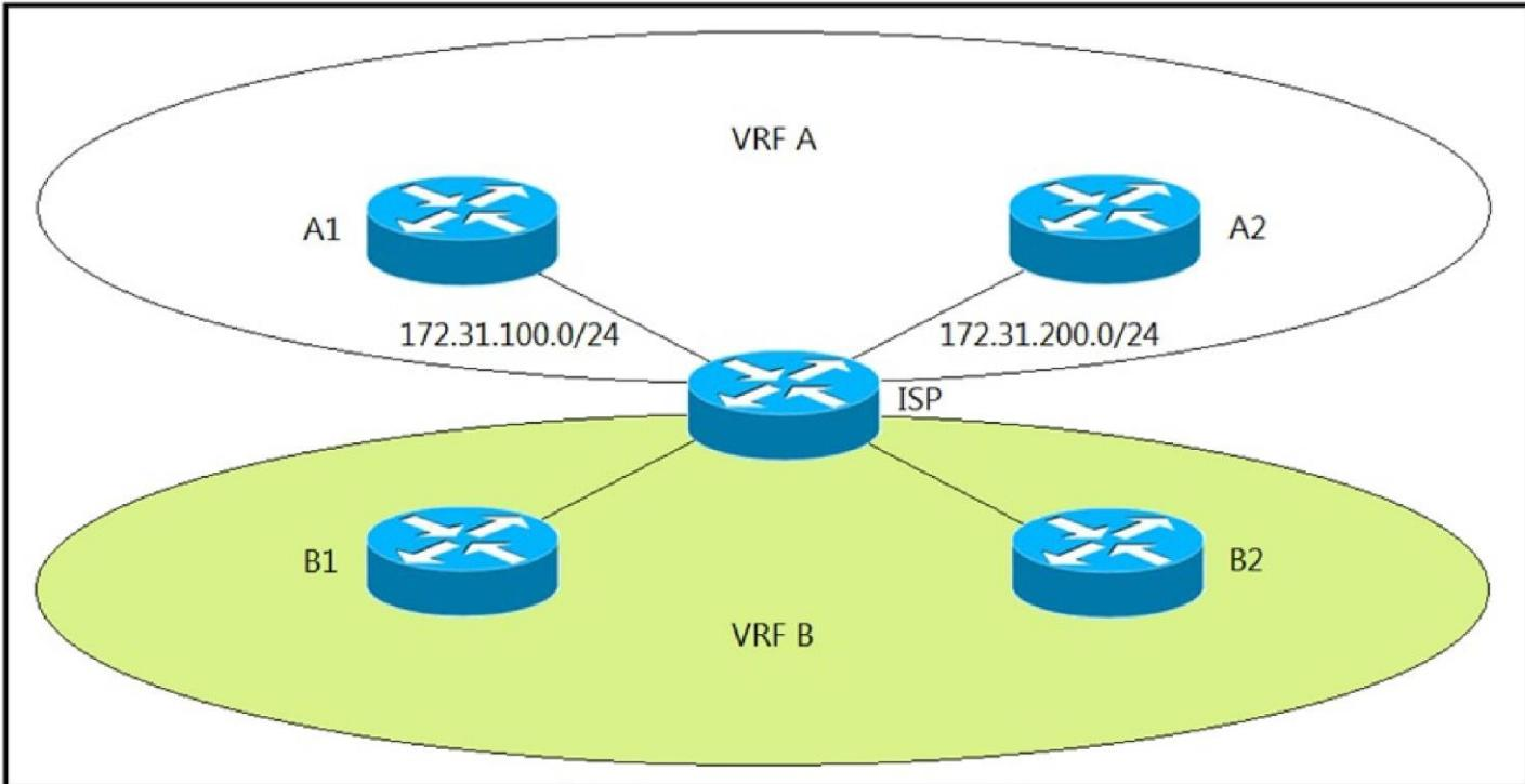
Refer to the exhibit. The ISP router is fully configured for customer A and customer B using the VRF-Lite feature. What is the minimum configuration required for customer A to communicate between routers A1 and A2?
