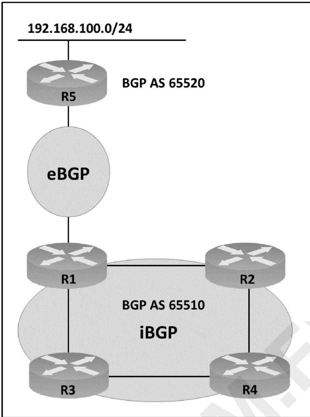
AS65510 iBGP is configured for directly connected neighbors. R4 cannot ping or traceroute network 192.168.100.0/24.
